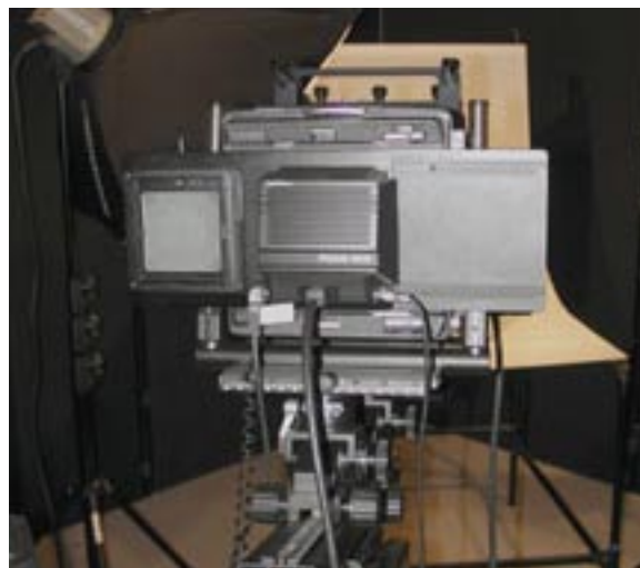
Sliding back to allow viewing while using medium format back on 4x5 camera.
