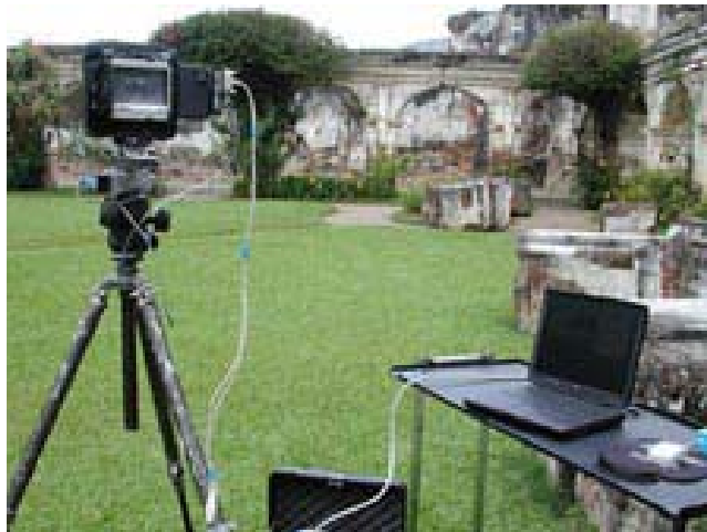
Left: Betterlight digital panoramic equipment on location in Antigua. Right: a section of the resulting panorama from using the large format digital panoramic system.
